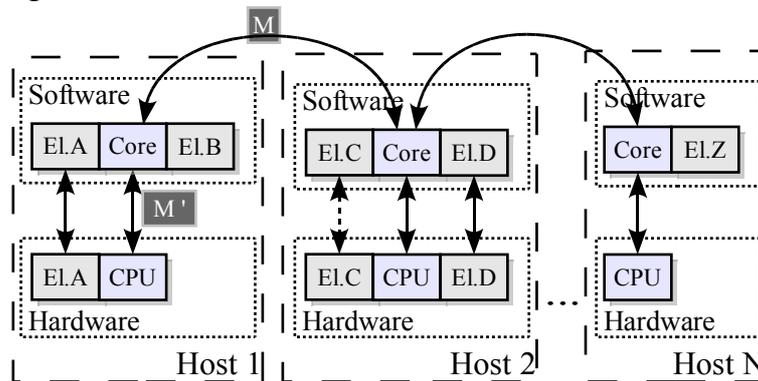
Fig 5 Cross-section of the architecture of a multiuser system for geometric modeling
