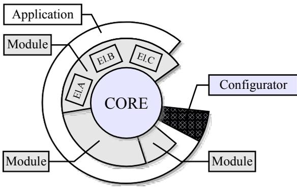
Fig 2 Structure of an open system for geometric modeling
